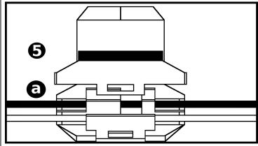
**{ILLUS. 5.a }** First insert the black and white 22 gauge wire into the widest end of a connector so that it fits snugly in the space provided. It will go all the way through the connector, and continue to the next light.
