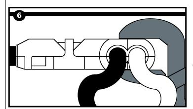
**{ILLUS. 6}** Squeeze the T connector closed using a pair of pliers on both ends of the connector.
