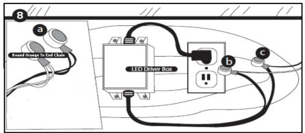
{ILLUS. 8} When all lights are installed, cap the ends of the 22 gauge wire separately with the round orange connectors. Caution: Do not connect the ends together as this will short out the system.
